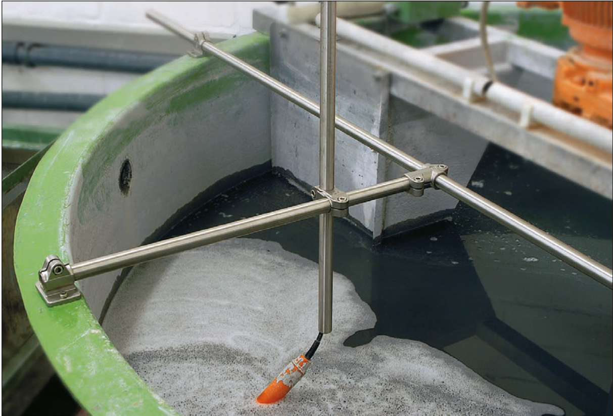
Simple probe fixation in an aggressive environment.
