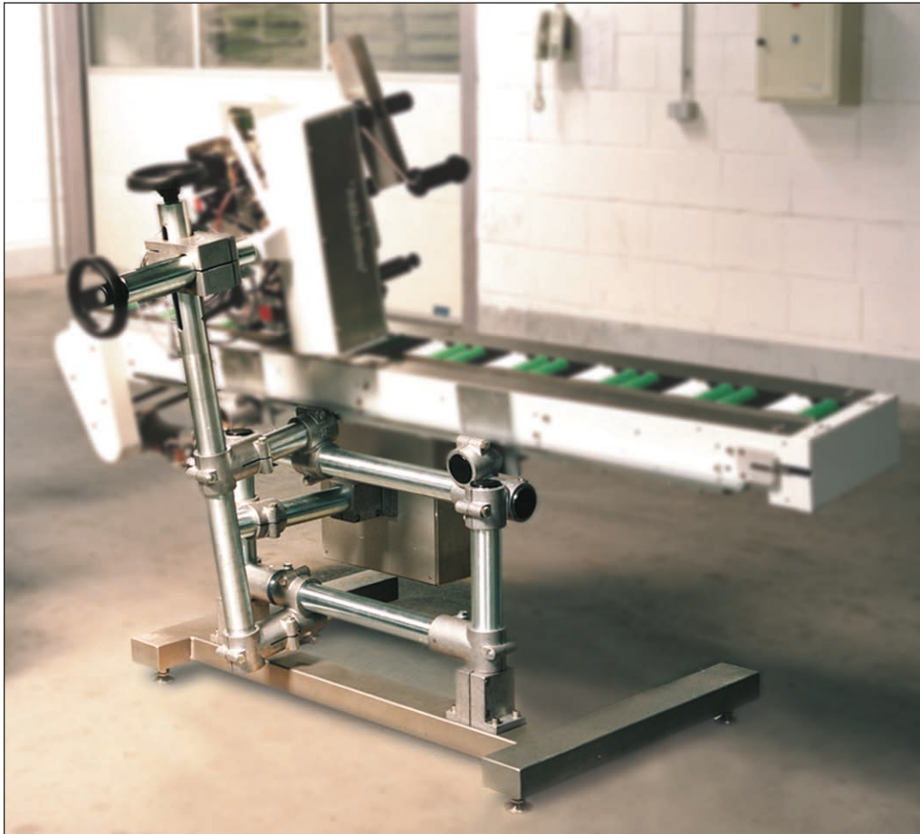
Frame for a labelling machine.
