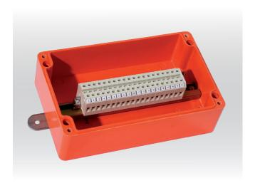
In case of fire protection not only rolling stock, but also railway application equipment has to fulfill special demands. For tunnel systems ROSE offers a range of E 30 enclosures acc. to DIN 4102 part 2. These enclosures are one part of the entire system for safety in tunnel systems in case of fire. E30 means that the complete electric system withstands the fire for 30 minutes for passenger evacuation.
