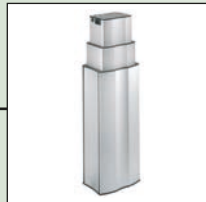
RK Powerlift telescope Hub max: 650 mm Fd max: 1.600 N Fz max: 800 N Vmax: 30 mm/s
