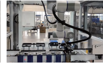
Battery Testing Loading and Unloading
